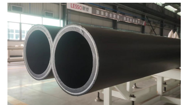
RTP 柔性輸氫複合管 RTP Flexible Hydrogen-transporting Composite Pipes
